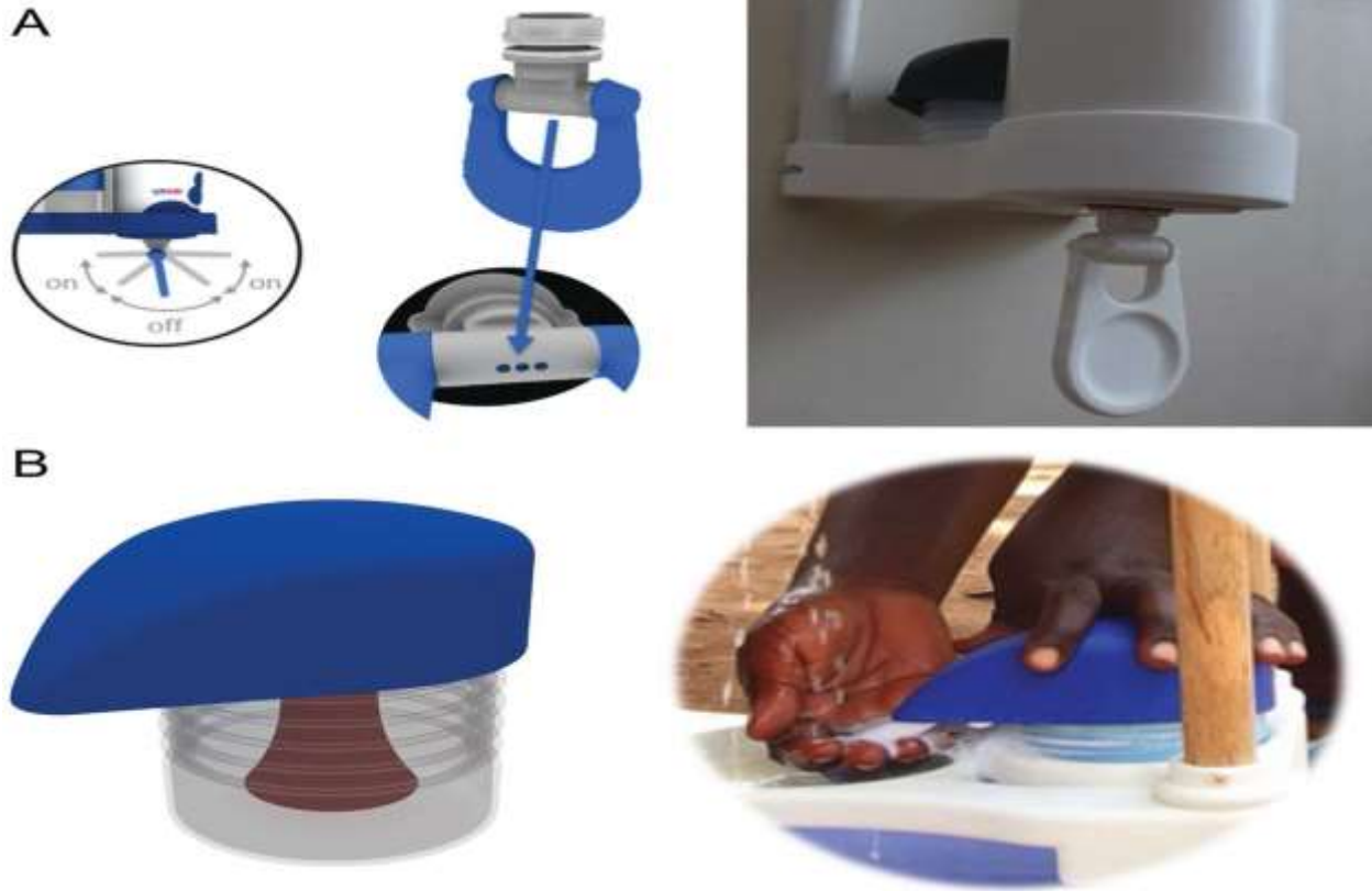
Water- and Soap-Dispensing Elements of the Povu Poa Handwashing
