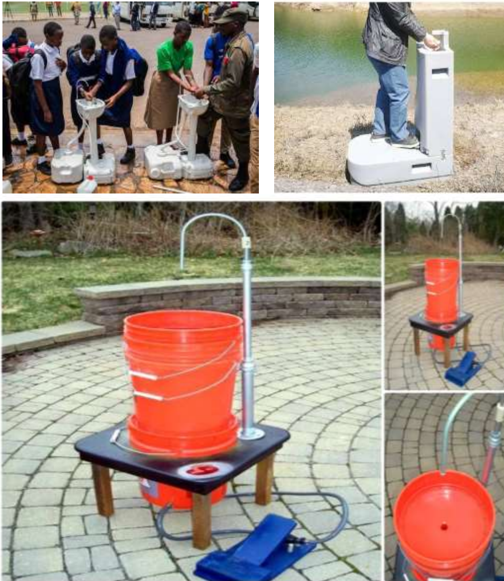
Various types of foot pump powered hand washing stations collated from various sources. Source: Scroll.in (top left) Toppla Group (top right),Instructables.com(bottom three)
