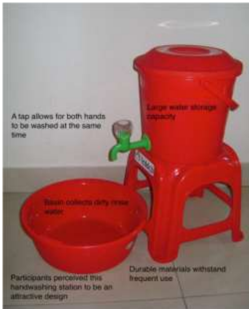
Simple kitchen bucket handwashing unit
